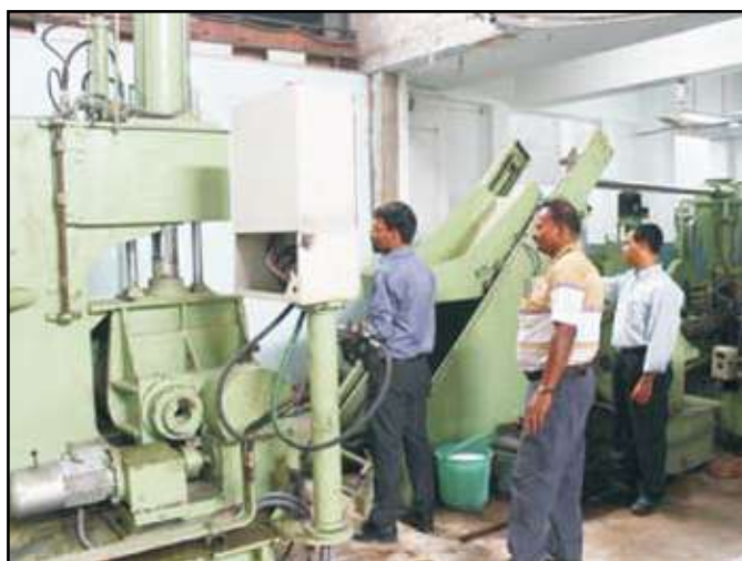
Kneader Extruder machine (50 Kgs)
