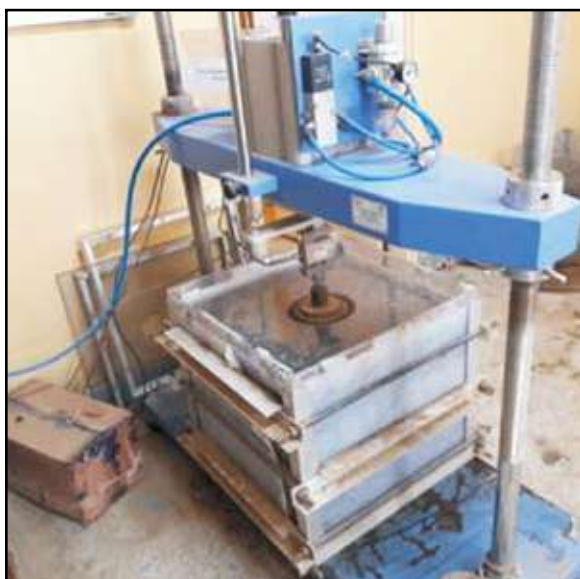
Actual Photograph of Pavement Model Testing on Cyclic Loading Equipment
