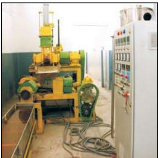
Kneader –Extruder machines installed at IJIRA(7 kgs)
