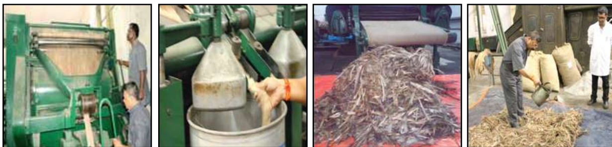
Trials on Biochemical Softening of Hard Root Cuttings of Jute at IJIRA Pilot Plant (No. of trials conducted: 16)
