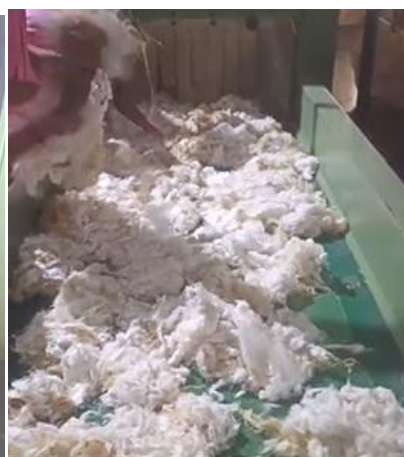
Blow room processing of cotton-bamboo blends
