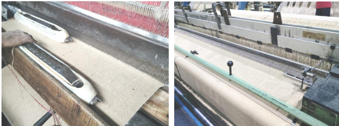
Preparation of DW Canvas and Hessian Fabric from Jute-Sisal blended yarn
