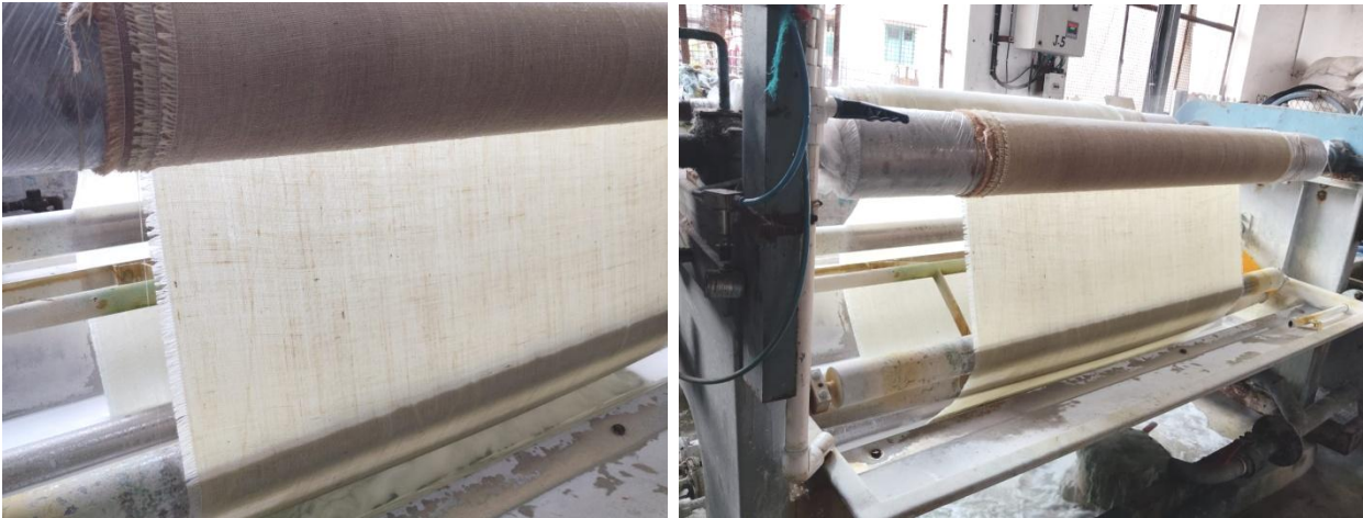
Bleaching and Softening of the Jute-Sisal blended fabric
