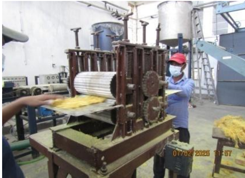
9 roller machine under fabrication based on satisfactory performance of 3 roller prototype machine with servo motor drive
