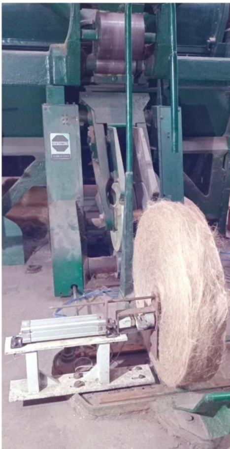
Automatic weight & MR% measurement in Pneumatic Controlled Roll Former
