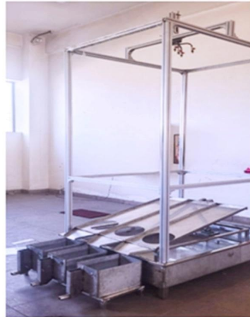
Rain Splash Experiment Apparatus for Soil (ASTM D 7101-07)
