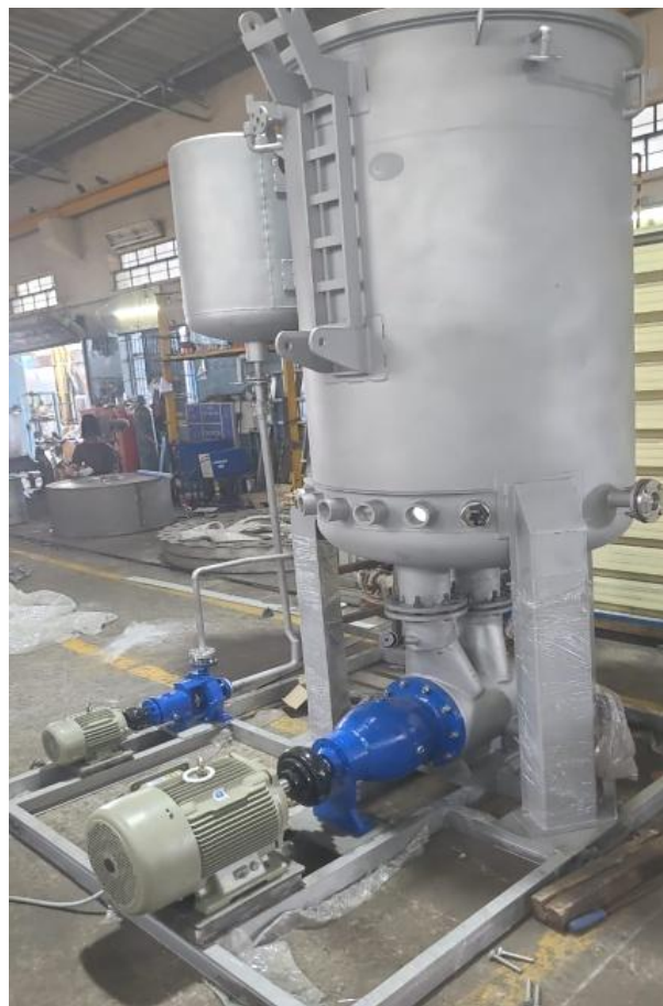
HT-HP Decorticating Machine (100 kg capacity)
