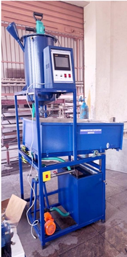
Sedimentation Retention Apparatus for Soil (As per ASTM D 5141-23)
