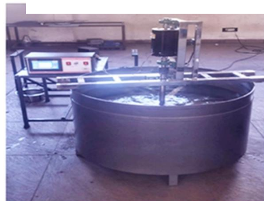
Shear Stress Experiment Apparatus for Soil (As per ASTM D 7207-05)
