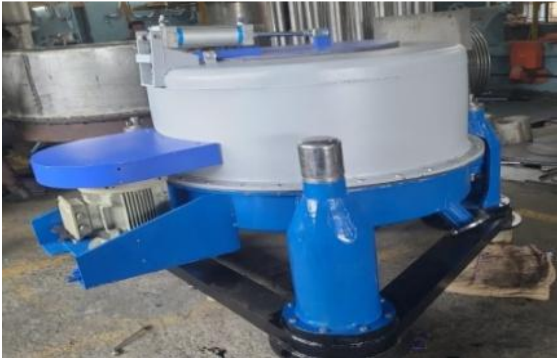
Hydroextractor (100 kg capacity)
