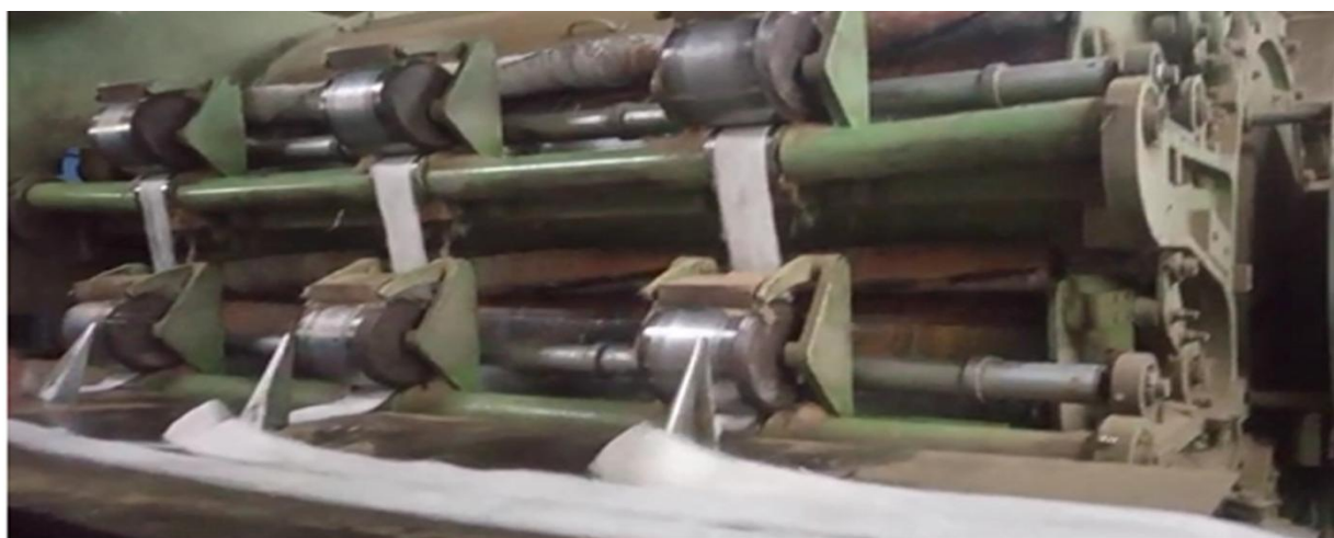
Processing of Ramie Fibre in 5X Card
