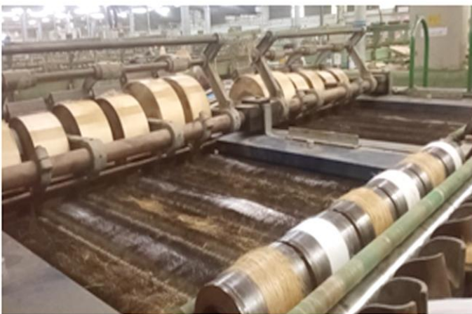
Mixing of Hackled Ramie and Flax top in open gill bar drawing
