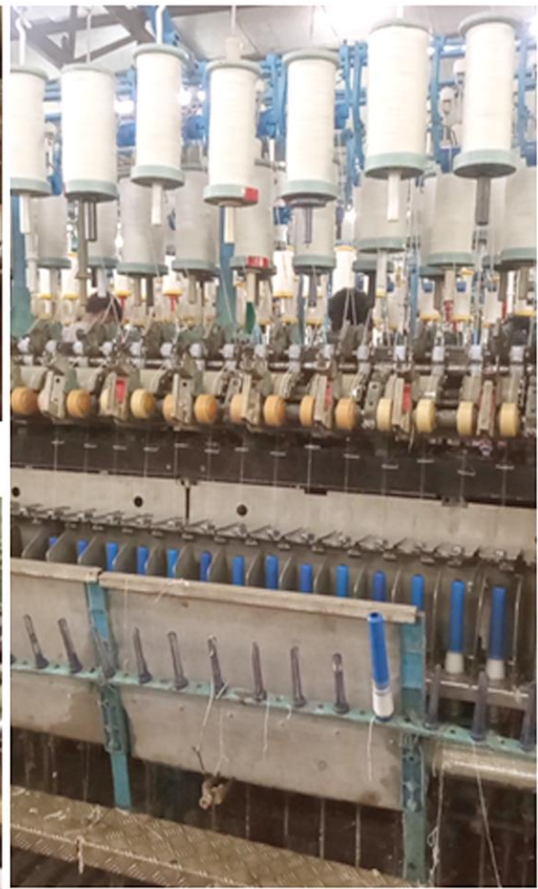
Wet Spinning of Ramie - Flax (50:50) blended yarn
