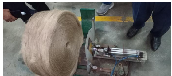
Online roll weight and moisture detection
