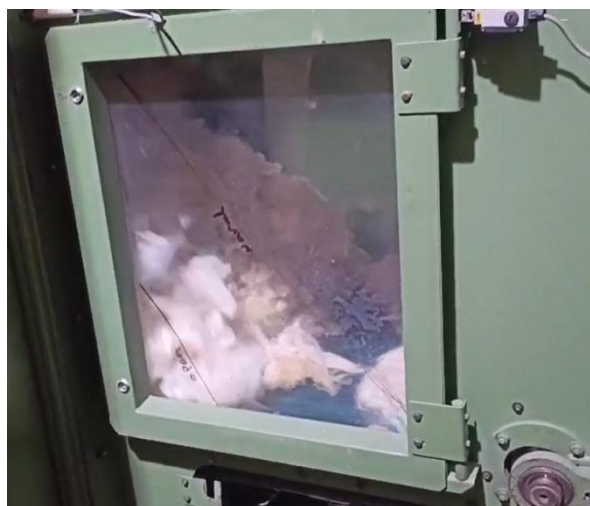
Cotton-Bamboo blending process in Blow-room
