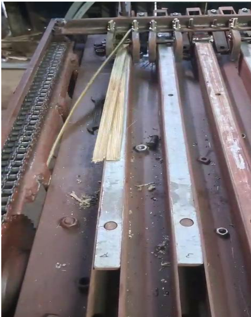
Multi-cutter bamboo stripping machine
