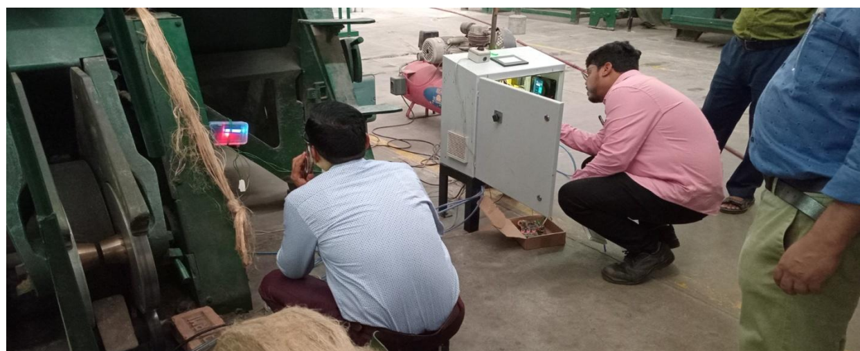
Demonstration of sliver length measurement on Pneumatically Controlled Roll Former
