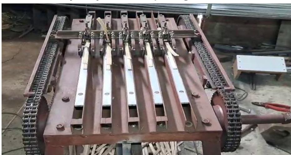
Bamboo Splitting Machine in Action
