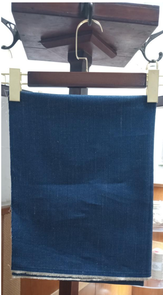
Denim woven with light jute-blended weft yarn
