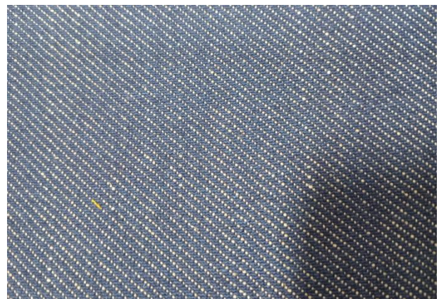
Denim woven with light jute-blended weft yarn
