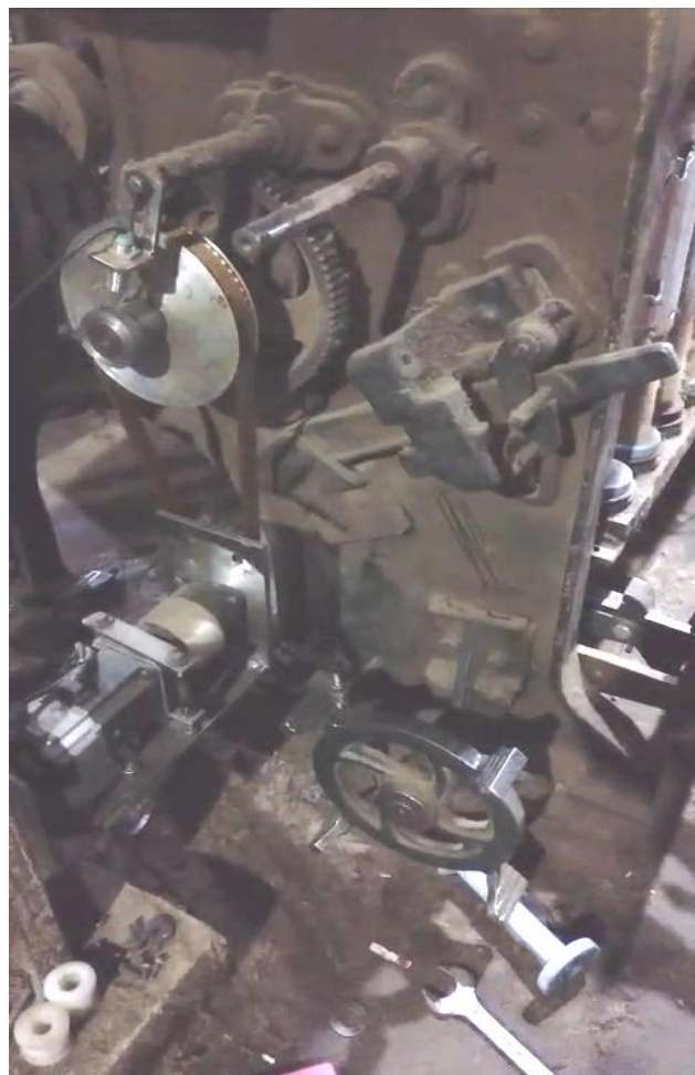
Auto doffing retrofit being implemented in a mill
