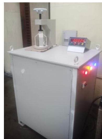
IJIRA Developed Ball Bursting Machine
